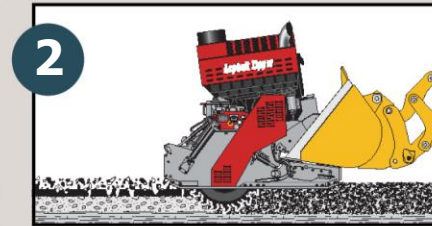
Pulverize old road surface and blend with base.
